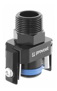
NPT male thread **Technology** Operating pressure Vacuum capability 3/4" MNPT PPS Grip Concept 0 to 232 psi -29 inHg (vacuum 98%) **Temperature** Construction Highlight Meets standards -4°F to +176°F Pipe and fittings: aluminum ASME B31.3 REACH Scalable system
